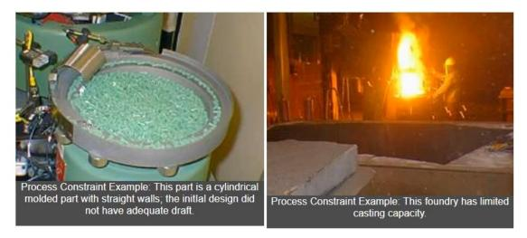
Another example involves a steel foundry. A foundry cannot pour or cast a part larger than its furnace capacity. The size of the furnace places a constraint on the mass of the part design. In this case, the team would need to decide whether the furnace size is going to be considered as a constraint to the design.
